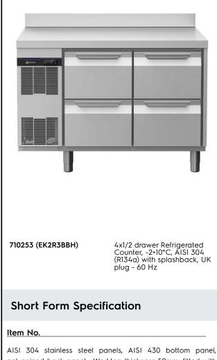
also 504 stainless steel panels, AISI 450 bottom panel, galvanized back panel. Worktop thickness 50mm, fitted with integrated rear splashback h=100mm. N. 4X1/2 drawers. Builtin refrigeration unit. Operating temperature: -2+10°C. R134a gas in refrigeration circuit.
